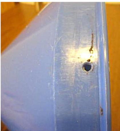
Drill three 3mm holes in the funnel edge close to the top rib, spaced at 120 degrees. (Use the baffle assembly rig to mark the spacing.)
